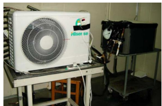
Fig. 21 Hybrid air conditioner outdoor unit with storage.
